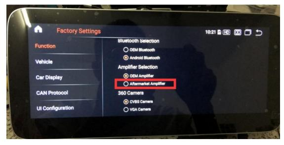
No sound for OEM system after installation
