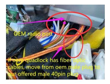
If all other has sound, Bluetooth phone call and navigation via android screen not have, then need install the external speaker: disconnect the 4 small plugs on power plug (2 blue 2 white), connect the white one with label(小喇叭) with the small speaker, another white plug connect to the blue plug that fits, left one blue plug empty
